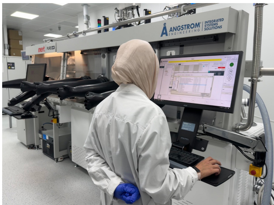
Pic. 7. Postdoctoral fellow Dr Gulzhan Bizhanova operates a thin-film deposition system for the fabrication of photovoltaic devices.
