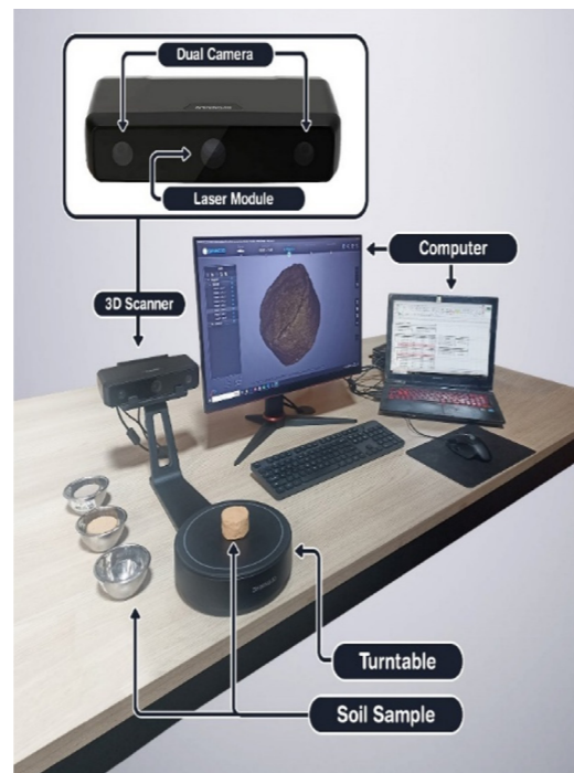
3-D Scan for Soil Volume Measurement
