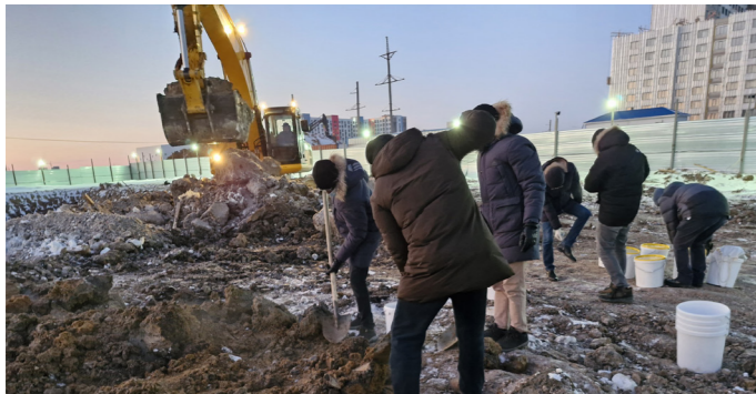
Picture 2. Extracting soil samples from a construction site in Astana
